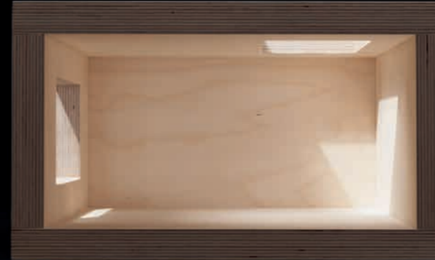
Combining the two openings creates a diversified lighting environment with variations in daylight intensity, a greater perception of space and more viewing options.
