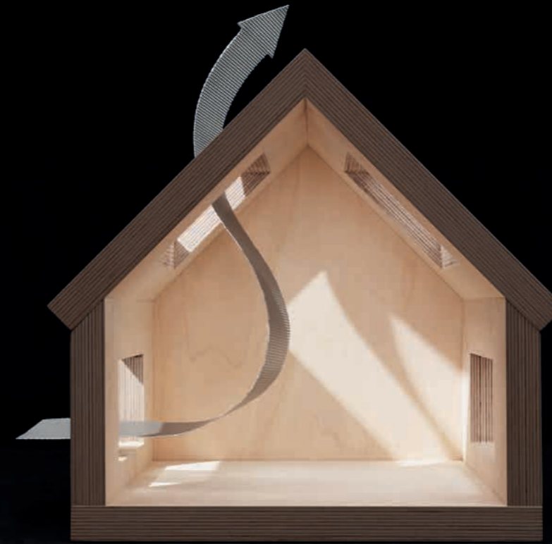
Natural ventilation with stack effect uses high-placed openings in combination with lower-placed openings, e.g. on the ground floor, to increase the buoyant warm air properties and flush the indoor environment within minutes.
