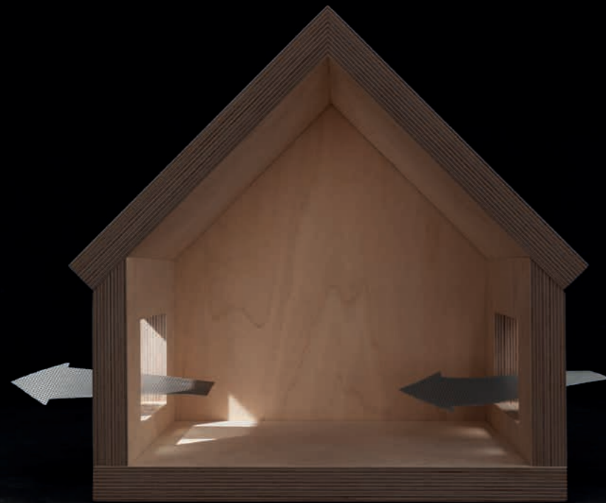
Cross-ventilation uses two or more open windows opposite each other to ventilate the room, exploiting different air pressure zones on both sides of the building to create a self-supporting air current.
