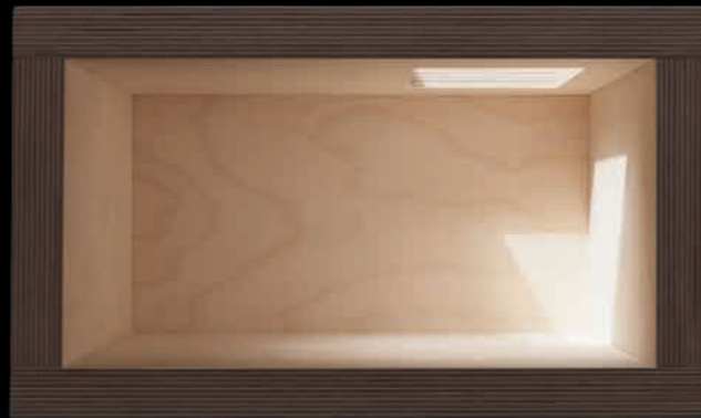
A horizontal opening through the roof provides intense daylighting in central or deep areas.
