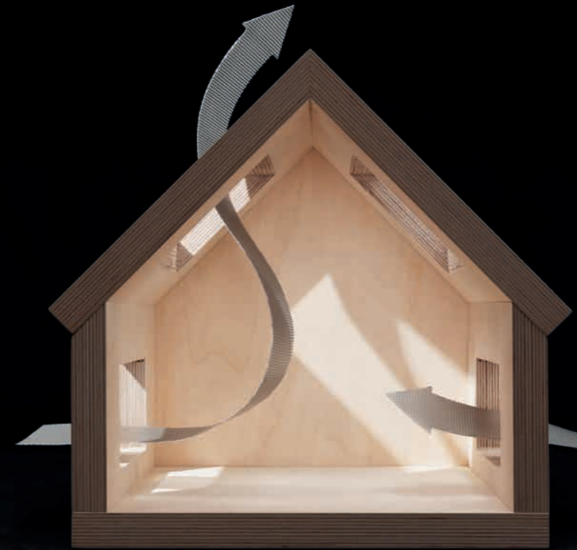
Opening the home in one or more places helps to lower the inside temperature without any mechanical support. Natural ventilative cooling is especially effective during the night.
